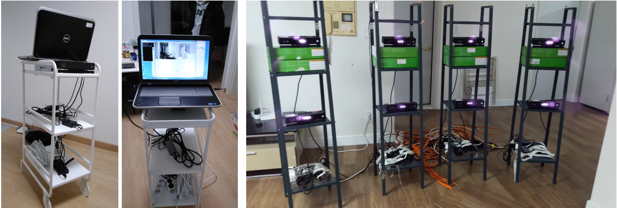
Systems for data acquisition: camera on moving cart (left), multiple Kinect v2 cameras (right)
